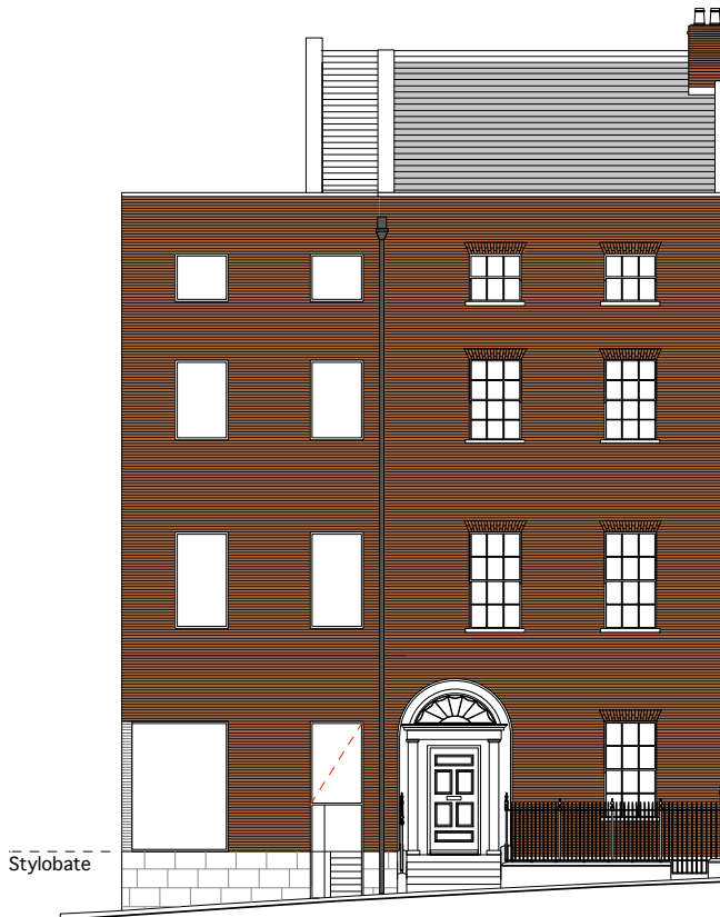
Diagram 1. Proposed front elevation showing continuation of flat brick wall and openings of same proportion as no. 15. In addition the idea of 'stylobate' is continued at the base level, continuing the ground floor datum. The placement of the 'shop door' is positioned in the 2nd. bay which is probably the original position of the main door.
