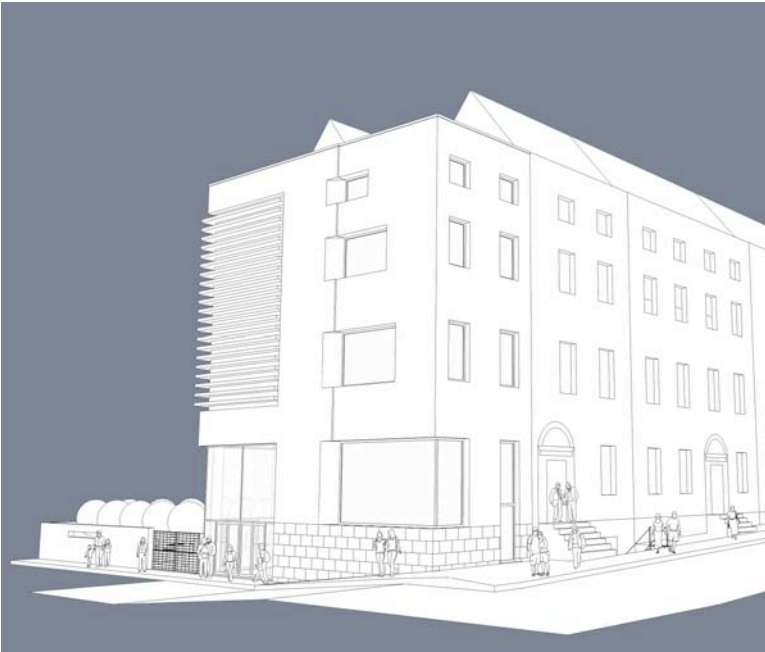
Diagram 6. View of the proposed scheme on Henrietta Street. The idea of stylobate or base is continued in the scheme and the missing 'brick wall' of the facade is re-instated with the new front facade of the new building.
